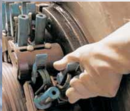
The handle lever is pressed together and the plug-in brush holder is slowly drawn from the holding fixture.
