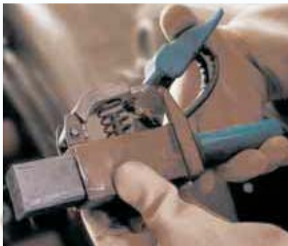
Changing and checking of the brush are carried out in safety – outside of the running motor.
